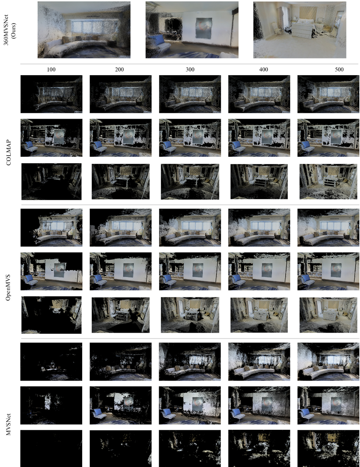
Figure 3: Comparisons of the results with different numbers of cameras. We show three scenes reconstructed using our method and other methods (COLMAP [2], OpenMVS [1], and MVSNet [3]). For each compared method, we show the reconstructed point cloud using different numbers of images in each row.
