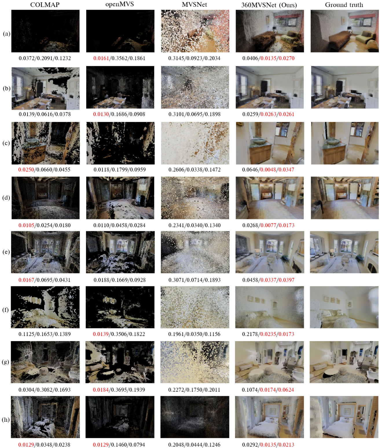
Figure 2: Results of equal-effort qualitative comparison. We use 25 360° images for scene (a), (h) and 49 360° images for scene (b)-(g). We convert the equirectangular images into cubemaps as the input images for COLMAP[2], OpenMVS[1], and MVSNet[3]. In total, for compared methods, we use 150 images for scene (a), (h) and 294 images for scene (b)-(g). We show the scores of accuracy/completeness/overall quality underneath each method’s result (lower is better) and mark the best result in red. Our method achieves the best completeness and overall scores across all examples.
