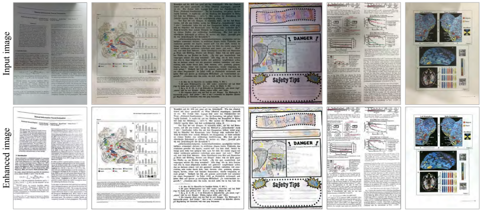
Figure 1: Photometric distortion correction. Our method is effective for correcting complex photometric distortions in document images. The top row shows the images captured by cameras, and the bottom row shows the enhanced images produced using the proposed method, which corrects shadows, shading, and color shift simultaneously.
