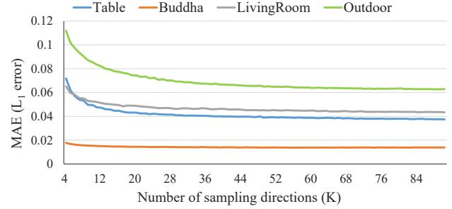
**Figure 6:** We show the relationship between the number of sampling directions and the accuracy of the recovered depth map, measured by the mean absolute error (in meter). Using more sampling directions could give more accurate results, at the cost of higher computational cost. We typically use 8 – 24 sampling directions per pixel.
