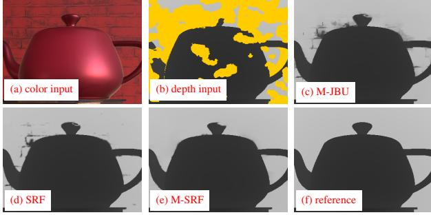
**Figure 8:** (a) and (b) show a case of missing regions with similar foreground and background color. Our multi-resolution approach (e) can reduce the texture copy artifacts compared to the single resolution one (d). It is worth noting that although M-JBU [RSD\*12] also runs in a multi-resolution manner, it still suffers from texture copy artifacts due to the insufficient background data inside the filter window, as shown in (c).
