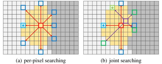
**Figure 3:** We sample lines to search for the representative pixels. (a) At each pixel with an invalid depth value (marked yellow), we uniformly sample a few directions for searching the best representative based on a similarity measurement. In this case, the neighbor labeled with a light blue asterisk is selected. (b) We stratify the sampling directions of adjacent pixels to search for different directions.
