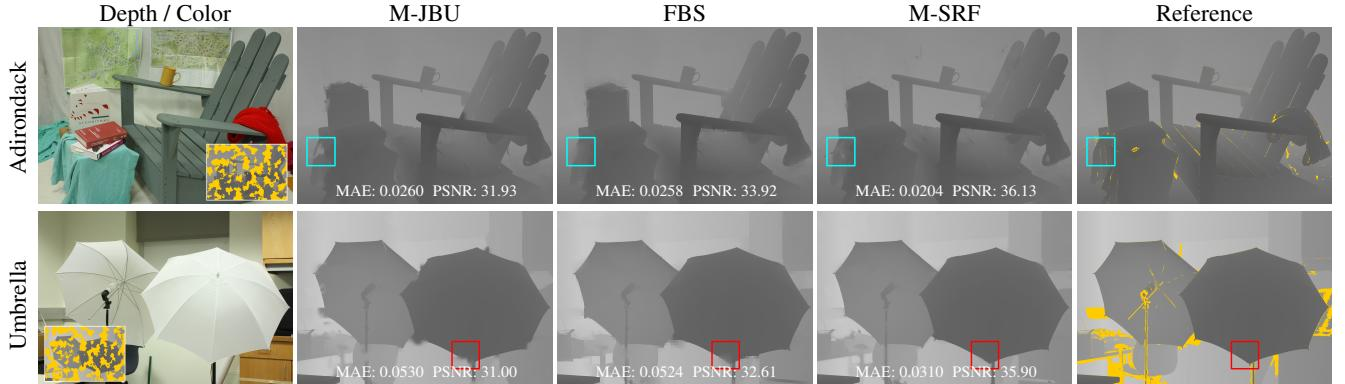
**Figure 12:** Comparisons of the Adirondack and Umbrella scenes in Middlebury 2014 data set [SHK\*14]. We allocate 20 milliseconds for M-JBU and M-SRF. The unoptimized FBS takes about 1.2 to 2.0 seconds. Our method can better preserve the depth discontinuities and achieve lower MAE and higher PSNR than M-JBU and FBS.
